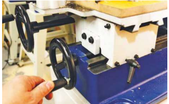
▲ The front to back adjustment is altered with this large wheel
